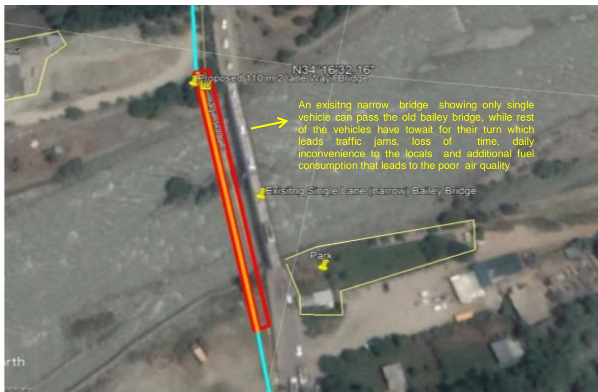
6 Figure 7.1: Map showing existing temporary bailey bridge which was designed for the single vehicle to pass through it.
